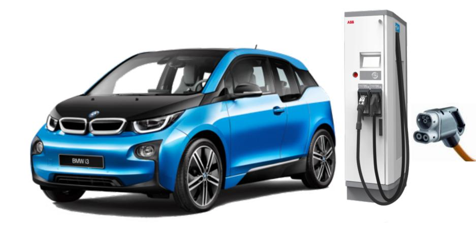
Rapid Charging: 30-45 minutes, now with the 'CCS' connector standardised. 50kW / 150kW / 350kW
